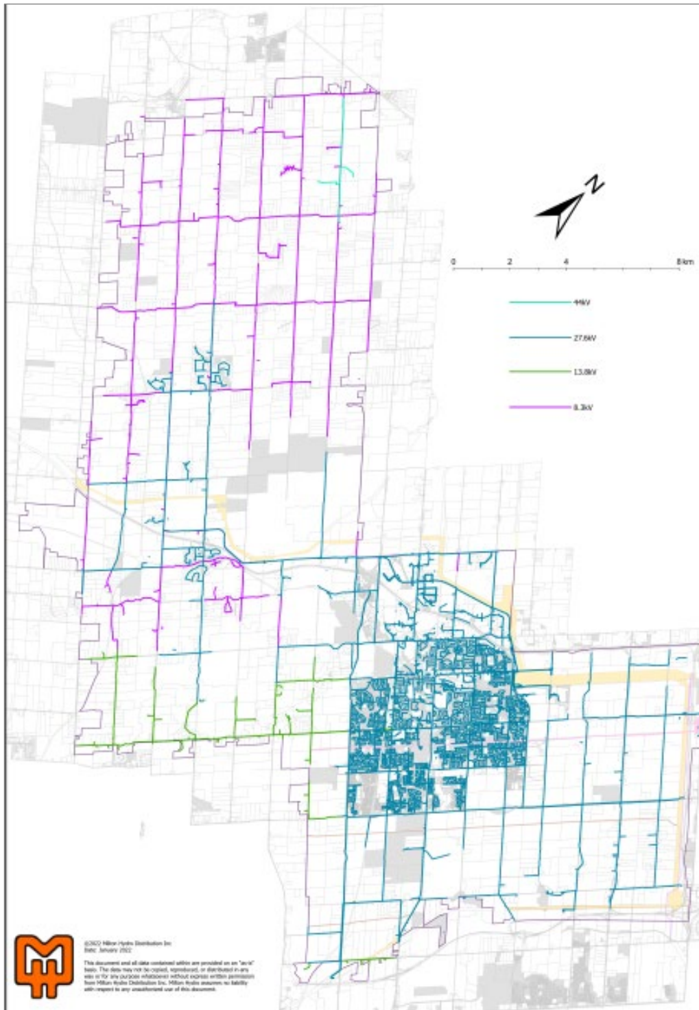
Figure 11 – Primary Distribution System by Voltage Rating
