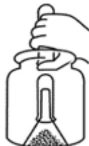
5. Mark the text tube at the water line with a rubber band.
